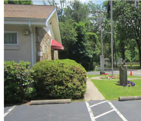
A rain garden can be installed on either side of the entrance to capture stormwater from the rooftop by redirecting the downspout under the sidewalk. Pervious pavement can replace sections of parking spaces to capture a large portion of the parking lot runoff. A preliminary soil assessment suggests that more soil testing would be required before determining the soil's suitability for green infrastructure.
